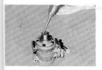
APPLY COMPRESSOR OIL TO INNER BORE
