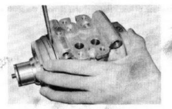
(b) Using a hammer and punch, remove the front housing by tapping on the protrusion.
