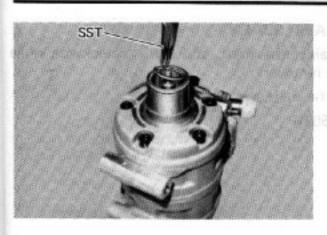
2. REMOVE CIRCLIP
