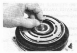
(c) Remove the shims from the shaft.
