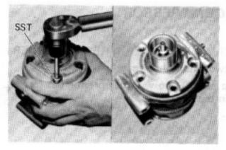
4. INSTALL FRONT HOUSING ON FRONT CYLINDER AND TIGHTEN SIX THROUGH BOLTS
