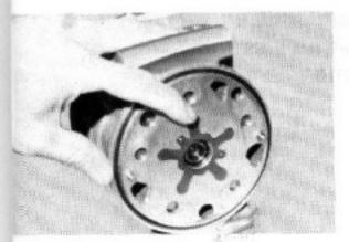
(c) Install the rear suction valve over the pins on the rear cylinder.
