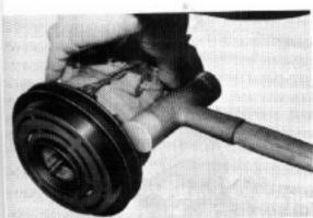
(b) Using a plastic hammer, tap the rotor off the shaft.
