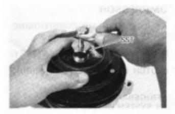
(b) Using SST and socket, remove the pressure plate. SST 07112-71010
