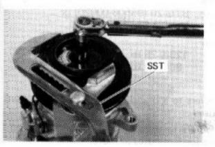
(b) Using SST and a torque wrench, install the shaft nut. SST 07110-77011
