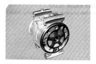
(d) Install the rear valve plate together with the discharge valve over the pins on the rear cylinder.
