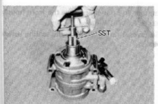
(b) Pull up the bar of the remover, and remove the shaft plate.
